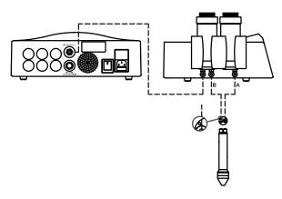
3. Fill with micro-crystal the container #2 without exceeding the line. The cap thread must be completely clean of micro-crystal. Is recommended to use #120 particle size micro-crystal.
